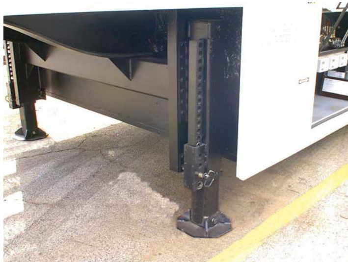
Figure 15: Front Stabilizing Legs and Auxiliary Support Legs
