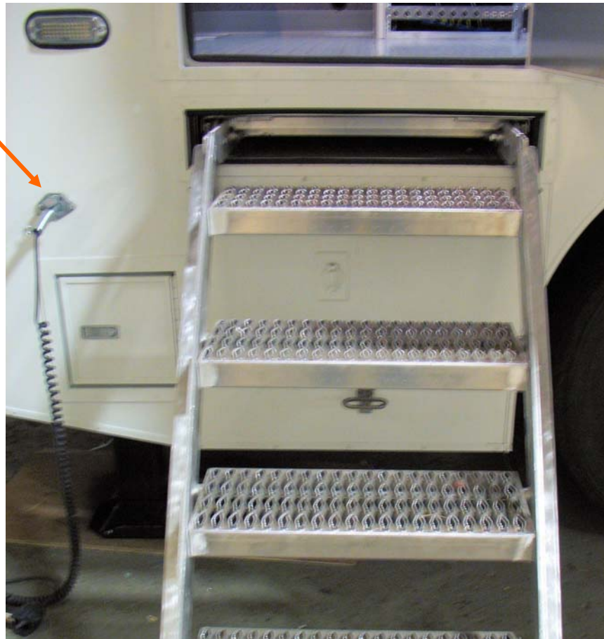
Figure 19: Slide-out Pendant Receptacle
