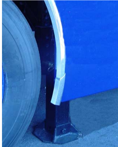
Figure 12: Rear Leveling Legs
