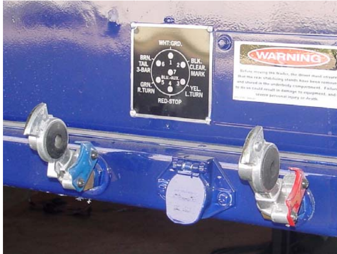
Figure 8: Glad Hand Connections
