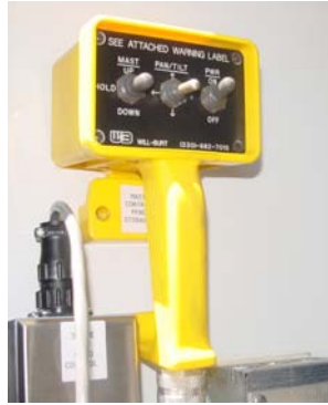
Figure 21: Mast Control Pendant
