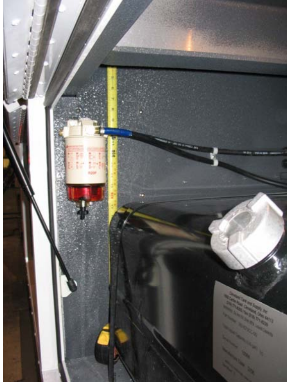
Figure 8. Filter with Reference from Compartment Ceiling
