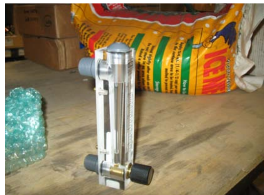
H1002405 – Flow Meter – Obsolete – GE Heat Exchanger, Primary Glycol Loop
