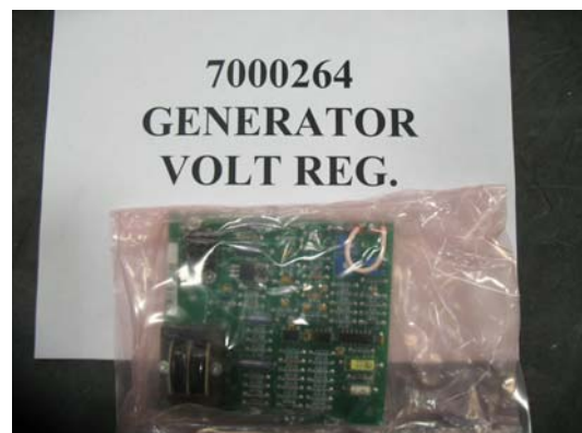
7000264 – Generator Voltage Regulator
